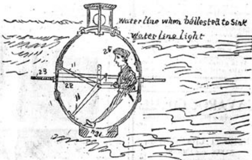
AMIDSHIPS SECTIONS OF THE HUNLEY SUBMARINE. From Sketches by W. A. Alexander.
